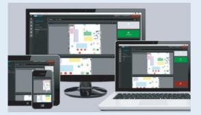
With Fleet Manager by MiR, you can **control multiple AMR units**. This web-based software centralizes critical AMR conditions, including battery status and current location, ensuring seamless workflow management. Fleet Manager also acts as a traffic controller, resolving conflicts and preventing traffic deadlocks by coordinating the movement of AMRs on designated paths, ensuring smooth operation.
